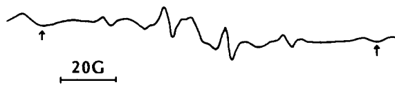
Figure 2 ESR spectrum of photoirradiated PMMA at 77 K in vacuum. Irradiation wavelength, 260 nm. Total photon fluence, 9.8 \times 10^{19} photons/cm 2 . Arrows indicate the doublet ( \cdot\text{CHO} ).
